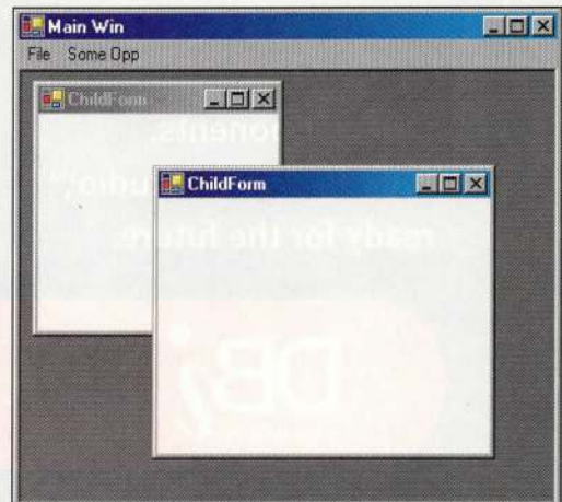
Figure 2 Create the MDI Application. You can create as many child windows as you like, hosted in the main parent frame window. Note that the child window menu is merged with that of its parent.
