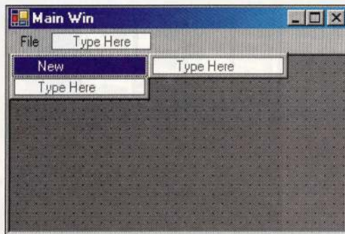
Figure 1 Build the Menu of the Main Frame's Parent Window. The Windows Forms visual designer lets you build menu items, then map them to handling methods. Windows Forms merge a child window's menu automatically in its MDI parent's menu.
